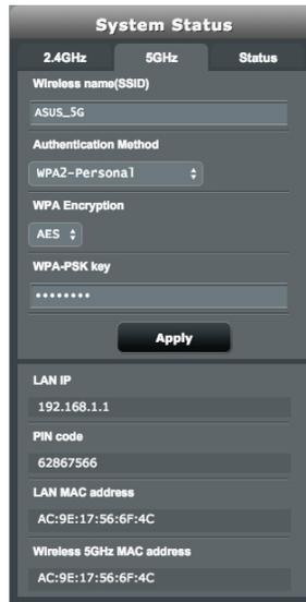
The screenshot shows the 'System Status' screen with the '5GHz' tab selected. The 'Wireless name(SSID)' field contains 'ASUS\_5G'. The 'Authentication Method' is set to 'WPA2-Personal'. The 'WPA Encryption' is set to 'AES'. The 'WPA-PSK key' field is filled with seven asterisks. Below these settings is an 'Apply' button. At the bottom, there are fields for LAN IP (192.168.1.1), PIN code (62867566), LAN MAC address (AC:9E:17:56:6F:4C), and Wireless 5GHz MAC address (AC:9E:17:56:6F:4C).
