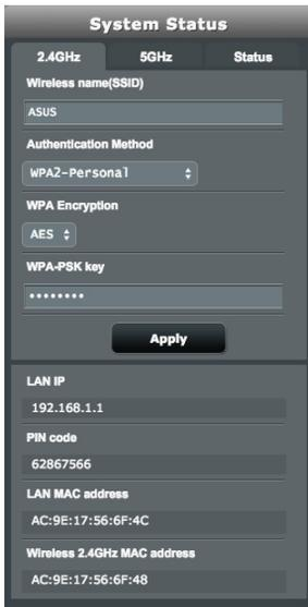
The screenshot shows the 'System Status' screen with the '2.4GHz' tab selected. The 'Wireless name(SSID)' field contains 'ASUS'. The 'Authentication Method' is set to 'WPA2-Personal'. The 'WPA Encryption' is set to 'AES'. The 'WPA-PSK key' field is filled with seven asterisks. Below these settings is an 'Apply' button. At the bottom, there are fields for LAN IP (192.168.1.1), PIN code (62867566), LAN MAC address (AC:9E:17:56:6F:4C), and Wireless 2.4GHz MAC address (AC:9E:17:56:6F:48).
