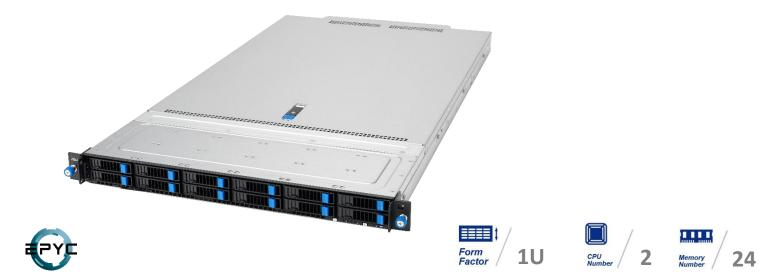
ASUS RS700A-E13 series is a server powered by AMD 9005 processors that supports up to 24 DIMMs, 4/12 NVMe, four expansion slots and dual M.2 and ASUS ASMB12-iKVM.
