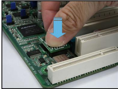
4. When installed, the board appears as shown.
