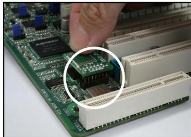
3. Press the board firmly until it is completely seated in place.
