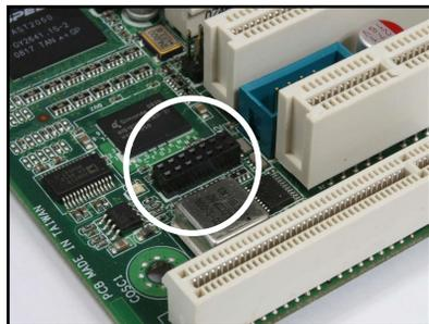
2. Place the board on the BMC connector of the motherboard, aligning with the pin connectors.
