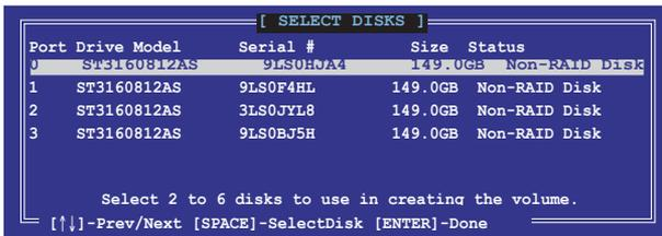
5. Use the up/down arrow key to select a drive, and then press <Space> to select. A small triangle marks the selected drive. Press <Enter> after completing your selection.
