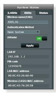
3. On the **Wireless name (SSID)** field, key in a unique name for your wireless network.
