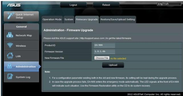
The Firmware Upgrade tab allows users to upgrade the firmware of the EA-N66 by uploading the firmware file.
