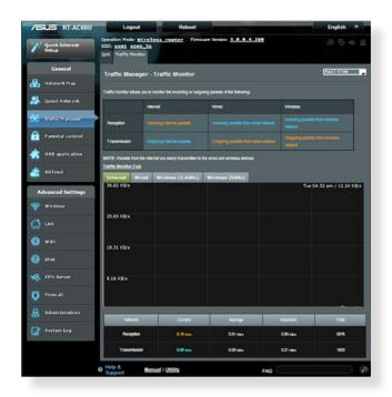
**NOTE:** Packets from the Internet are evenly transmitted to the wired and wireless devices.
