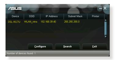
**NOTE:** When you set the router to Access Point mode, you need to use Device Discovery to get the router's IP address.
