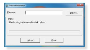
**IMPORTANT:** Launch the rescue mode on the router before using the Firmware Restoration utility.
