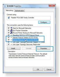
To obtain the IPv4 IP settings automatically, tick Obtain an IP address automatically.
