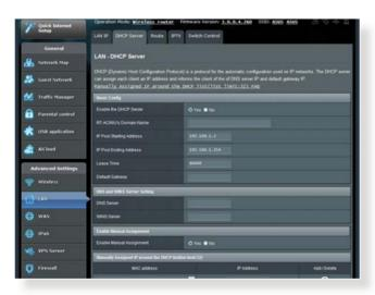
SSID has been hidden. If your device can find SSIDs from other routers but cannot find your router's SSID, go to Advanced Settings > Wireless > General, select No on Hide SSID, and select Auto on Control Channel.
