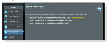
**NOTE:** Network printer utility is supported on Windows® XP, Windows® Vista, and Windows® 7 only. To install the utility on Mac OS, select **Use LPR protocol for sharing printer**.
