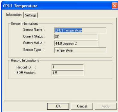
4. Click the **Settings** tab to adjust the sensor threshold values. Click on the up/down arrow button after each threshold value to adjust. Click **OK** to close the window.
