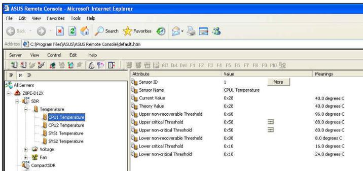
The **Detail/SEL** window displays the sensor data attributes, values, and meanings. From this window, you can adjust the sensor threshold values by clicking the up/down arrow button after each value.
