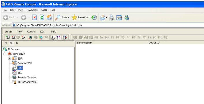
2. Click before the **FRU** to display available FRU information, then click before the module/component. Select a module or component from the list to display the FRU information in the **Detail/SEL** window.
