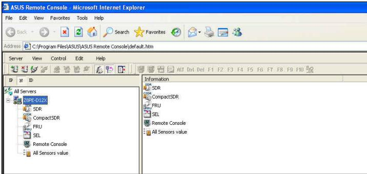
2. Click **+** before the **SDR** to display the sensor groups (e.g. Temperature), then click **+** before a sensor group to display the individual sensors. Select a sensor (e.g. CPU1 Temperature) to display its values in the **Detail/SEL** window.
