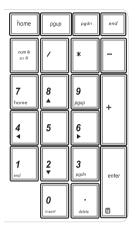
A numeric keypad is available on selected Notebook PC models. You can use this keypad for numeric input or as pointer direction keys.
