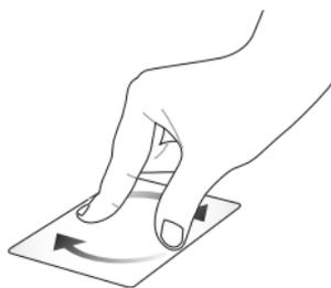
To rotate an image, place two fingers on the touchpad then turn one finger clockwise or counterclockwise while the other stays still.
