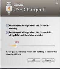
3. Move the slider to set the battery charge threshold to stop the USB Charger+ function.
