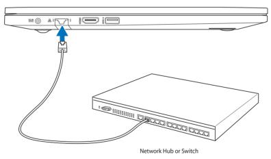
Network cable with RJ-45 connectors
