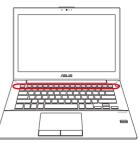
The Hot Key locations on the function keys may vary depending on model but the functions should remain the same. Follow the icons instead of the function keys.
