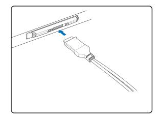
Carefully connect any cables or adapters needed by the PC card. Usually connectors can only be inserted in one orientation. Look for a sticker, icon, or marking on one side of the connector representing the top side.
