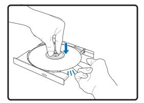
3. Hold the disc by the edge and face the disc's printed side up. Push down on both sides of the disc's center until the disc snaps onto the hub. The hub should be higher than the disc when correctly mounted.
