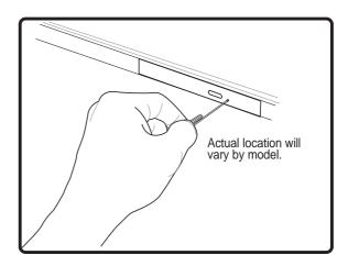
The emergency eject is located in a hole on the optical drive and is used to eject the optical drive tray in case the electronic eject does not work. Do not use the emergency eject in place of the electronic eject. Note: Make sure not to stab the activity indicator located in the same area.
