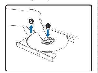
Eject the tray and gently pry the edge of the disc upwards at an angle to remove the disc from the hub.
