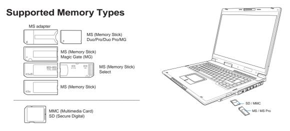
IMPORTANT! Never remove cards while or immediately after reading, copying, formatting, or deleting data on the card or else data loss may occur.
