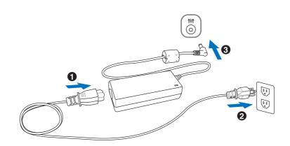
NOTE: This Notebook PC may come with either a two or three-prong plug depending on territory. If a three-prong plug is provided, you must use a grounded AC outlet or use a properly grounded adapter to ensure safe operation of the Notebook PC.
