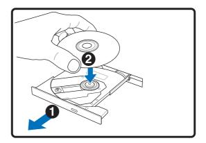
2. Gently pull on the drive's front panel and slide the tray completely out. Be careful not to touch the CD drive lens and other mechanisms. Make sure there are no obstructions that may get jammed under the drive's tray.
