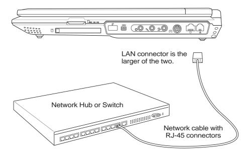
NOTE: The built-in modem and network cannot be installed later as an upgrade. After purchase, modem and/or network can be installed as a PC card (PCMCIA).
