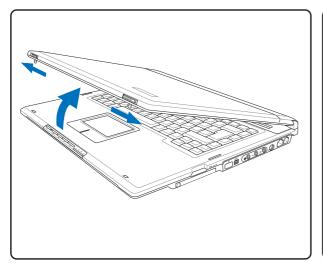
WARNING! When opening, do not force the display panel down to the table or else the hinges may break! Never lift the Notebook PC by the display panel! 4. Turn ON the Notebook PC
