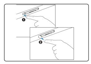
1. Press in the toggle eject button and release. The recessed spring loaded toggle button will extend when pushed in and released.
