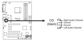
M2N-E SLI CPU Internal Audio Connector
