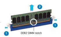
Remove the DIMM from the socket.
