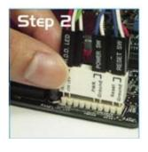
When installed, the Q-connector appears as shown.
