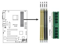
M2N-E SLI 240-pin DDR2 DIMM Sockets
