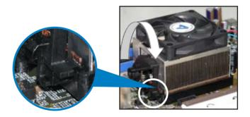
5. When the fan and heatsink assembly is in place, connect the CPU fan cable to the connector on the motherboard labeled CPU\_FAN.
