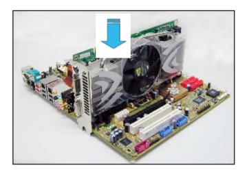
4. Insert the second graphics card into the other slot. Make sure that the card is properly seated on the slot.
