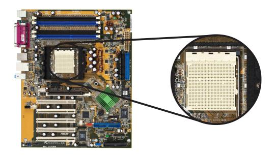
2. Unlock the socket by pressing the lever sideways, then lift it up to a 90°-100° angle.
