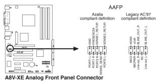
We recommend that you connect a high-definition front panel audio module to this connector to avail of the motherboard high-definition audio capability.
