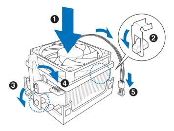
3. Align the other end of the retention bracket (near the retention bracket lock) to the retention module base. A clicking sound denotes that the retention bracket is in place.
