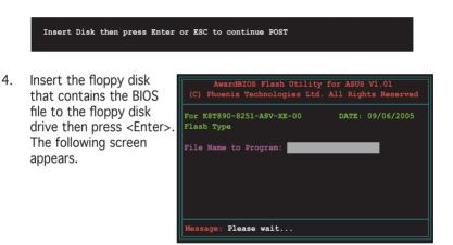
5. When the correct BIOS file is found, EZ Flash performs the BIOS update process and automatically reboots the system when done.
