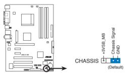
A8S-X SE Chassis Intrusion Connector
