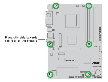
Before you install the motherboard, study the configuration of your chassis to ensure that the motherboard fits into it.
