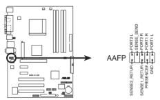
**A8S-X SE Analog Front Panel Connector**
