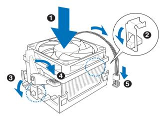
3. Align the other end of the retention bracket (near the retention bracket lock) to the retention module base. A clicking sound denotes that the retention bracket is in place.
