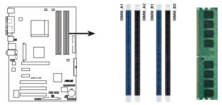
A8S-X SE 184-pin DDR DIMM Sockets
