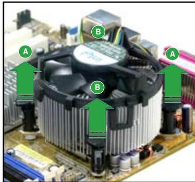
4. Remove the heatsink and fan assembly from the motherboard.
