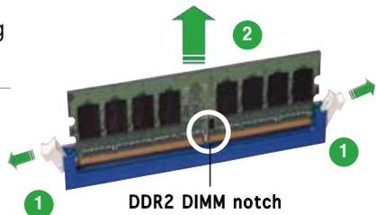
2. Remove the DIMM from the socket.
