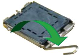
4. Lift the load plate with your thumb and forefinger to a 100° angle (A), then push the PnP cap from the load plate window to remove (B).
