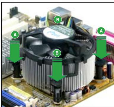
3. When the fan and heatsink assembly is in place, connect the CPU fan cable to the connector on the motherboard labeled CPU\_FAN.
