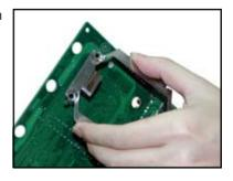
3. Press the upper spring hooks inward, then insert to the upper CPU heatsink holes until they snap in place.
