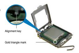
Close the load plate (A), then push the load lever (B) until it snaps into the retention tab.
