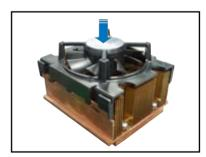
Use a Phillips screwdriver to tighten the four heatsink screws in a diagonal sequence.
