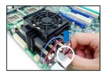
2. Grip the top cover clamps until the top cover hooks are released, then carefully lift the top cover while supporting the fan base with your free hand.
