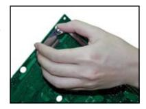
Press the lower spring clips inward, then insert to the lower CPU heatsink holes until they snap in place.
