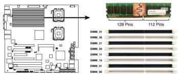
DSEB-DG Series 240-pin FB-DIMM sockets
