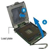
Position the CPU over the socket, making sure that the gold triangle is on the bottom-left corner of the socket. The socket alignment key should fit into the CPU notch
