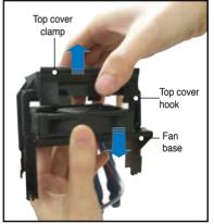
Position the fan base over the DIMMs, and insert the fan base legs into the FB-DIMM holes until the legs are securely in place.
