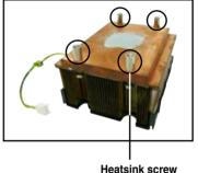
To install the CPU heatsink and fan:
