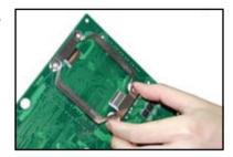
If you installed a second CPU, repeat steps 2 to 4 to install the CEK spring to the CPU2 heatsink holes.
