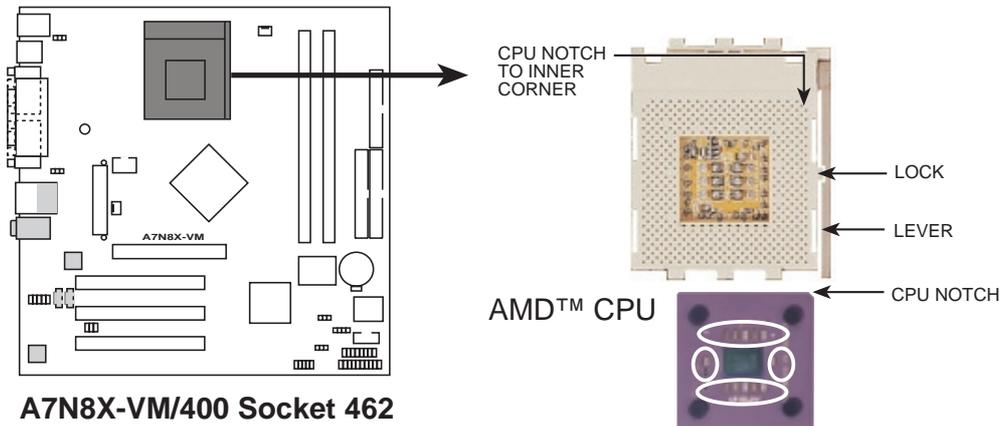
Each AMD CPU has a “marked” corner. This corner is usually indicated with a notch, and/or a golden square or triangle. Refer to this indicator while orienting the CPU. A fan and heatsink should be attached to the CPU to prevent overheating.
