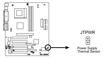
A7V266-C Thermal Sensor Connector
