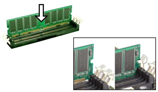
Unlocked Retaining Clip Locked Retaining Clip
