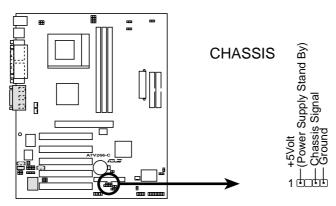
A7V266-C Chassis Open Alarm Lead
