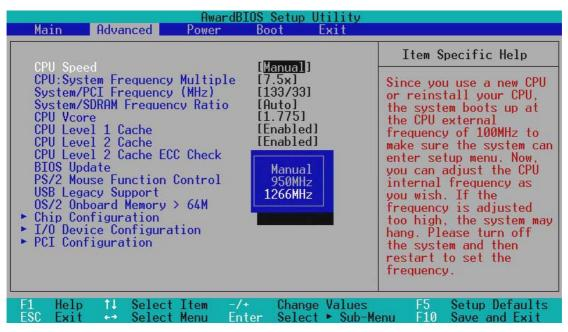
For processors with locked frequency multiplier
