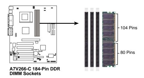
**WARNING!** Be sure that the DIMMs you use can handle the specified DDR RAM MHz or else bootup will not be possible.
