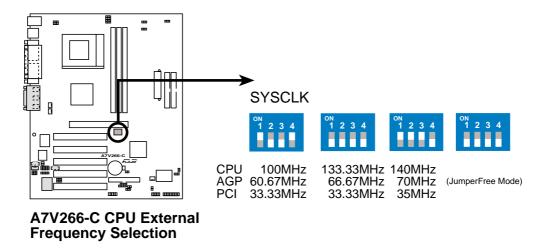
**WARNING!** Set the CPU frequency only to the recommended settings. Frequencies other than the recommended CPU bus frequencies are not guaranteed to be stable. Overclocking the processor is not recommended. It may result in a slower speed.
