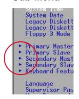
Note that a right pointer symbol (as shown in the left view) appears to the left of certain fields. This pointer indicates that you can display a sub-menu from this field. A sub-menu contains additional options for a field parameter. To display a sub-menu, move the highlight to the field and press <Enter>. The sub-menu appears. Use the legend keys to enter values and move from field to field within a sub-menu as you would within a menu. Use the <Esc> key to return to the main menu.
