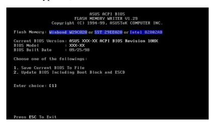
**IMPORTANT!** If the word "unknown" appears after **Flash Memory:**, the memory chip is either not programmable or is not supported by the ACPI BIOS and therefore, cannot be programmed by the Flash Memory Writer utility.
