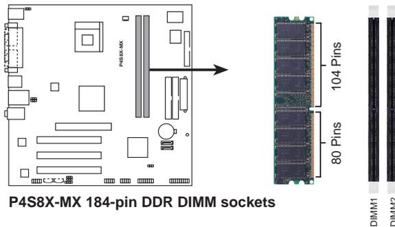
P4S8X-MX 184-pin DDR DIMM sockets
