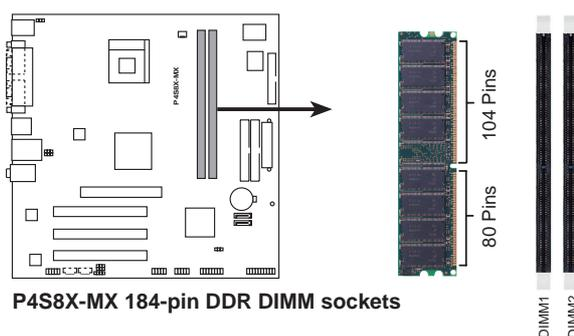
**P4S8X-MX 184-pin DDR DIMM sockets**
