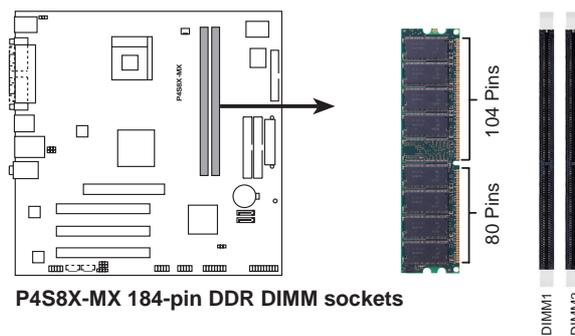
**P4S8X-MX 184-pin DDR DIMM sockets**
