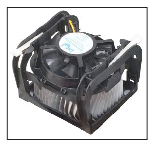
4. When the fan and heatsink assembly is in place, connect the CPU fan cable to the connector on the motherboard labeled CPU\_FAN1.
