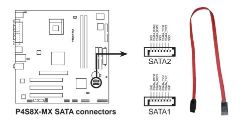
If you install SATA hard disk drives, you can create a RAID 0, RAID 1, or JBOD configuration with the SIS964 RAID controller. Refer to page 2-16 for the BIOS setting and page 3-18 for creating a RAID driver disk.
