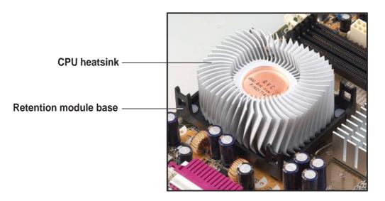
2. Position the fan with the retention mechanism on top of the heatsink. Align and snap the four hooks of the retention mechanism to the holes on each corner of the module base.
