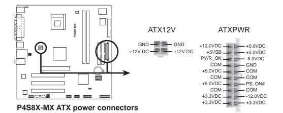
Make sure that your ATX 12 V power supply can provide 8 A on the +12 V lead and at least 1 A on the +5-volt standby lead (+5 VSB). The minimum recommended wattage is 230 W, or 300 W for a fully configured system. The system may become unstable and may experience diffculty powering up if the power supply is inadequate.
