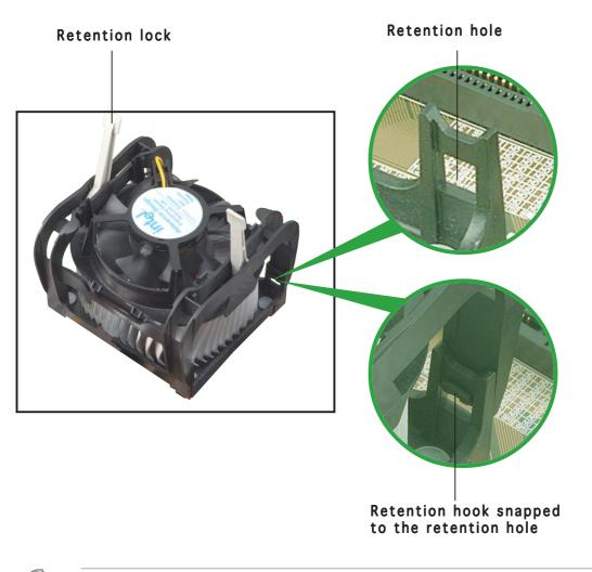
Keep the retention locks lifted upward while fitting the retention mechanism to the module base.
