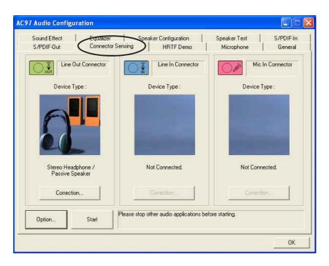
The Realtek® EZ-connection dialog box shows your current audio connections. The text at the bottom of the box explains your audio connection status. An *X mark* denotes an incorrect connection.
