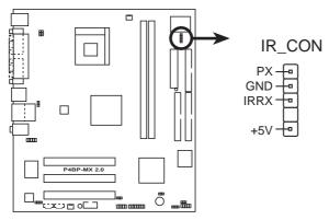
P4BP-MX 2.0 Infrared Module Connector
