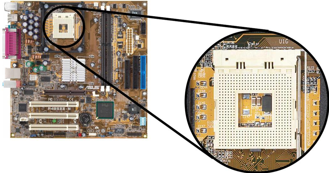
2. Unlock the socket by pressing the lever sideways, then lift it up to a 90°-100° angle.
