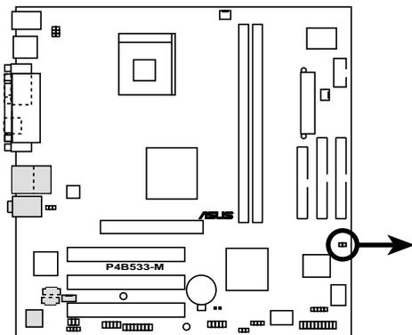
**TIP:** If the case-mounted LED does not light up, try reversing the 2-pin plug.
