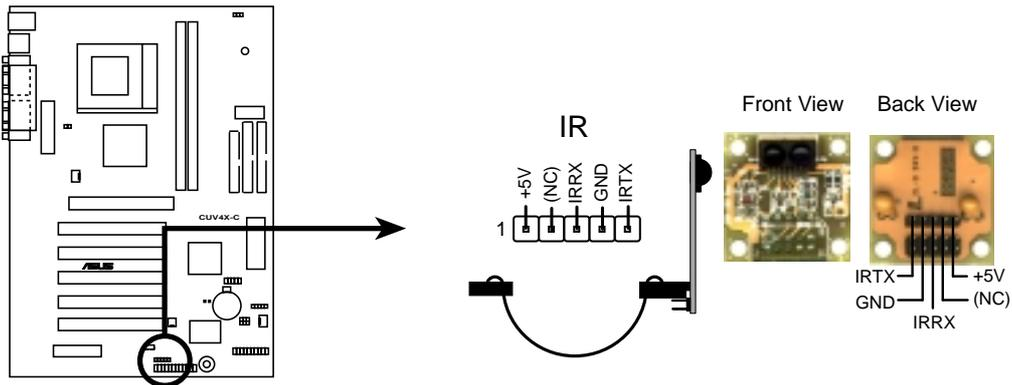
**CUV4X-C Infrared Module Connector**
