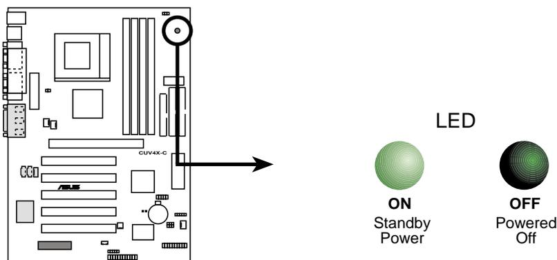
CUV4X-C Onboard LED
