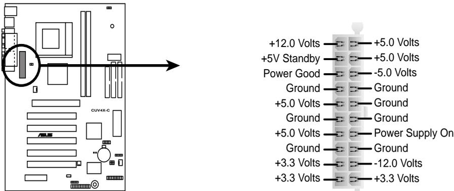
CUV4X-C ATX Power Connector
