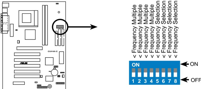
**CUV4X-C DIP Switches**
