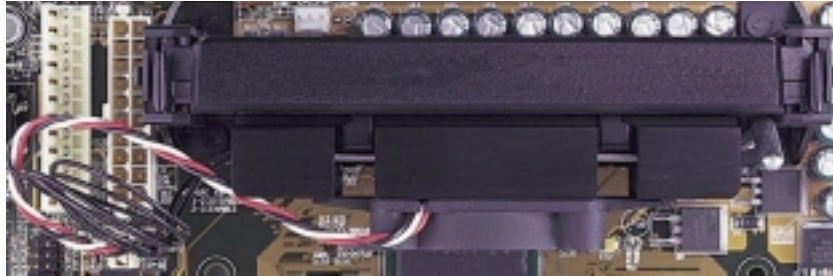
AMD Athlon™ processor with heatsink and fan (top view)
