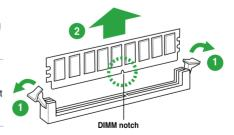
2 Remove the DIMM from the socket
