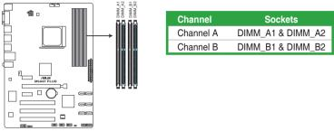
M5A97 PLUS 240-pin DDR3 DIMM sockets
