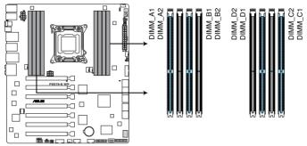
P9X79-E WS 240-pin DDR3 DIMM socket
