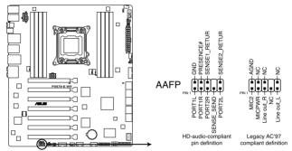
P9X79-E WS Analog front panel connector
