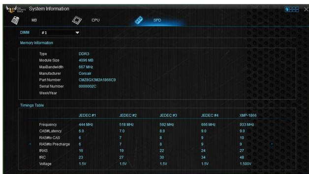
The screenshot shows the 'System Information' window with the 'SPD' tab selected. It displays memory information for DIMM #1, including type (DDR3), size (4096 MB), bandwidth (9.67 GHz), manufacturer (Corsair), and part/serial numbers. Below this is a 'Timings Table' with columns for JEDEC #1 through #4 and XMP-1686, listing various timing parameters like Frequency, CAS Latency, RAS#to CAS#, RAS#to Precharge, RAS#, RRC, and Voltage.
