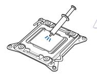
Apply the Thermal Interface Material to the CPU heatsink and CPU before you install the heatsink and fan, if necessary.
