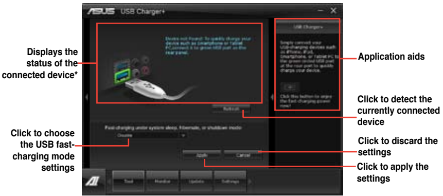
* The illustration above shows that no device connected to your PC for fast-charging.
