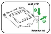
3. Lift the load lever in the direction of the arrow until the load plate is completely lifted.
