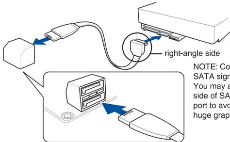
NOTE: Connect the right-angle side of SATA signal cable to SATA device. You may also connect the right-angle side of SATA cable to the onboard SATA port to avoid mechanical conflict with huge graphics cards.
