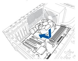
5. Place nine (9) screws into the holes indicated by circles to secure the motherboard to the chassis.
