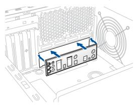
4. Place the motherboard into the chassis, ensuring that its rear I/O ports are aligned to the chassis' rear I/O panel.
