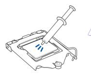
Apply the Thermal Interface Material to the CPU heatsink and CPU before you install the heatsink and fan, if necessary.
