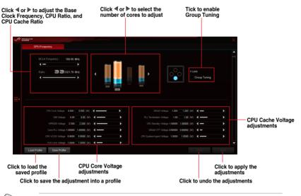
• Set the CPU Ratio Setting item in BIOS to [Auto] before using the CPU Frequency in TPU. Refer to the BIOS chapter of your motherboard's user guide for details.
