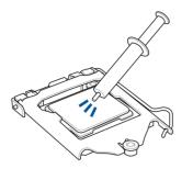
Apply the Thermal Interface Material to the CPU heatsink and CPU before you install the heatsink and fan, if necessary.
