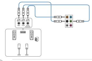
If you are using Windows 8.1 platform, use only the gray audio port for Side Speaker Out in a 6-channel configuration.
