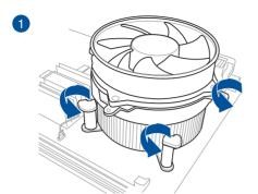
To uninstall the CPU heatsink and fan assembly
