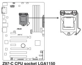
Ensure that you install the correct CPU designed for LGA1150 socket only. DO NOT install a CPU designed for LGA155 and LGA1156 sockets on the LGA1150 socket.
