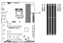
SABERTOOTH Z97 MARK 1 240-pin DDR3 DIMM socket
