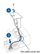
To install the 35 mm assistant fan on the cover hatch:
