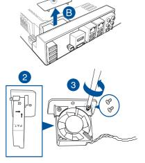
Align and insert the cover lid and the assistant fan assembly into the Thermal Armor and secure it with the screw that you removed in step 1.
