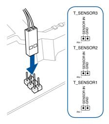
Put the thermistor sensor in contact with the surface of the component or part you want to monitor and secure it with an adhesive tape.
