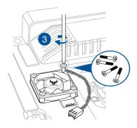
Connect the fan cable connector to the assistant fan (ASST\_FAN2) header on the motherboard.
