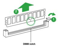
2. Remove the DIMM from the socket.
