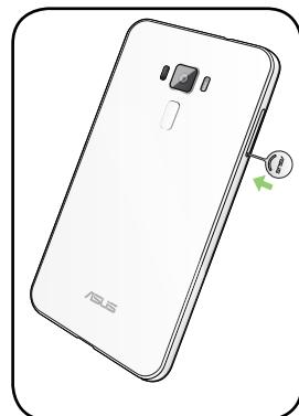
3. Remove the MicroSD card from the Nano SIM /MicroSD combo card slot.
