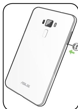
3. Remove the Micro SIM / Nano SIM card from the Micro SIM, Nano SIM / MicroSD combo card slot.
