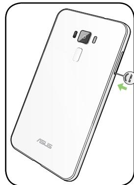
3. Insert the MicroSD card into the Nano SIM / MicroSD combo card slot.
