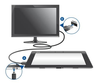
To connect an HDMI-compliant display:
