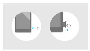
Remove the tray and place the micro SIM card inside it, with the angled corner fitting snugly into the angled corner of the tray.
