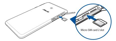
6. Put the micro-SIM/memory card compartment cover back in place.
