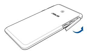
2. Press the memory card to eject, then pull it out.
