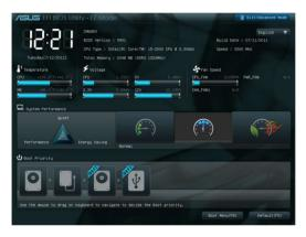
Click Exit/Advanced Mode on the right upper corner of the screen, and then select Advanced Mode. From the menu bar of the Advanced Mode screen, select Monitor.
