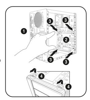
5. Push the the front panel cover slightly outwards, then set it aside.
