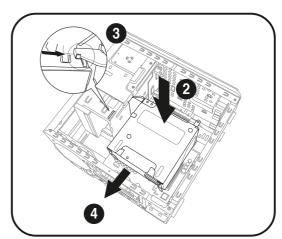
5. Secure the PSU with the screw you removed earlier.
