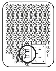
If the voltage supply in your area is 200-240V, set the switch to 230V.
