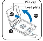
Position the CPU over the socket, making sure that the gold triangle is on the bottom-left corner of the socket. Fit the socket alignment key into the CPU notch.
