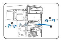
For SATA HDD: Connect the SATA signal and power plugs to the connectors at the back of the drive.
