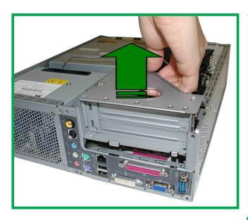
1. To remove the I/O cover from the chassis, pullout the expansion card assembly.
