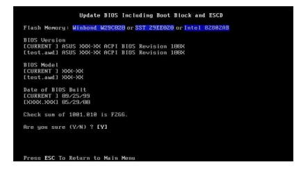
7. The utility starts to program the new BIOS information into the Flash ROM. The boot block is updated automatically only when necessary. This minimizes the possibility of boot problems in case of update failures. When the programming is done, the message *"Flashed Successfully"* appears.
