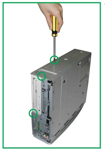
1. Remove the three screws on each marked location as shown. This frees the DVD/CD/HD drive assembly.
