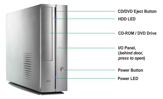
The front bezel door conceals the and features: a PCMCIA slot, 4-in-1 card slot, the fiber optical SPDIF in and out connectors, the 4 and 6-pin 1394 jacks, two USB connectors (Ports 2&3), headphone and microphone connectors
