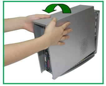
3. Open the case, lifting the top cover.
