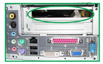
3. After removing the I/O cover, the back panel exposes the external I/O port to permit external access for component connections, like a modem card connector.
