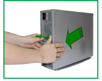
2. Separate the case and chassis cover: use your thumbs to pull it off, from the front to the back, then lift it off the chassis.
