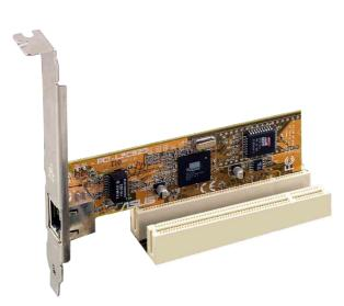
2. Align and firmly plug the PCI card into the slot.
