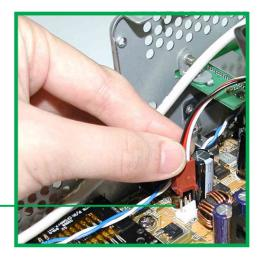
CPU fan connector – (CPU\_FAN1)
