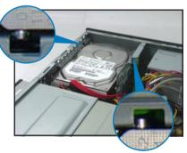
When the HDD screws align with the screw rails, push the drive carefully until it is completely flushed on the bay.
