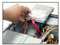
Place the HDD on the tray. Make sure that the HDD screws are aligned with the screw holes and rails.
