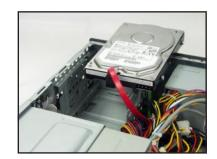
Connect the 15-pin SATA power plug from the power supply unit to the power connector at the back of the drive.
