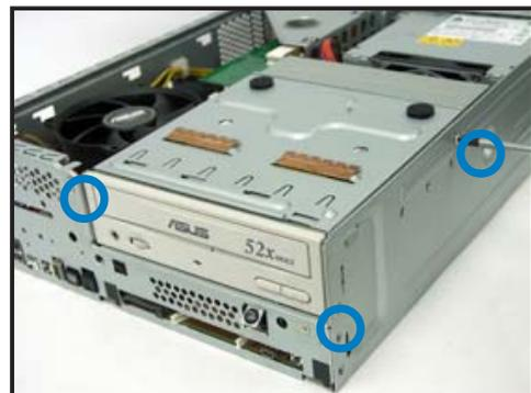
To install a **Serial ATA** hard disk drive:
