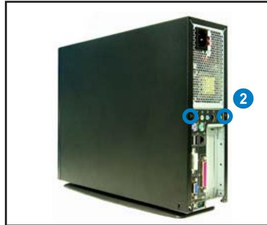
2. Use a Phillips (cross) screw driver to remove the cover screws. Keep the screws for later use.
